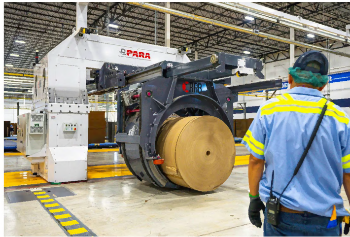
The Para Crab roll stock delivery system reduces product damage and improves plant safety.
